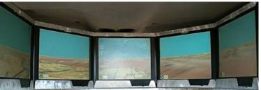
NASA remotely operated the SCOUT rover using SmartCam3D in a 5 panel configuration at Meteor Crater this week. The ACES advanced cockpit evaluation system was used for test and performed beautifully operating the vehicle over the course of several miles. The ACES uses SmartCam3D in a panoramic display mode which provides the operator with a 180 degree field of view.
