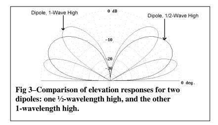
In the plots shown in Fig 3, the elevation angle above the horizon is represented in the same fashion that angles are measured on a protractor. The concentric circles are calibrated to represent ratios of field strengths, referenced to the strength represented by the outer circle. The circles are calibrated in decibels. Diminishing strengths are plotted toward the center.
