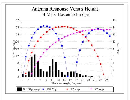
Fig 4—Elevation response patterns of three Yagis at 120, 70 and 35 feet, at 14 MHz over flat ground. The patterns are overlaid with the statistical elevationangles for the path from Boston to continental Europe over the entire 11-year solar sunspot cycle. Clearly, the 120-foot antenna is the best choice to cover the low angles needed, but it suffers some at higher angles.
