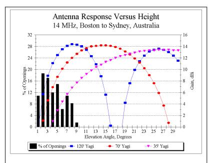
Fig 5—Elevation responses for same antennas as Fig 4, but for a longer-range path from Boston to Sydney, Australia. Note that the prevailing elevation angles are very low.
