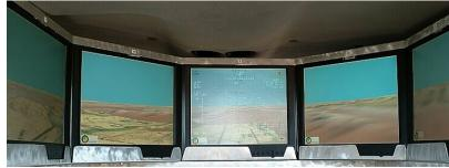
NASA remotely operated the SCOUT rover using SmartCam3D in a 5 panel configuration Crater this week. The ACES advanced cockpit evaluation system was used for test and beautifully operating the vehicle over the course of several miles. The ACES uses Smapanoramic display mode which provides the operator with a 180 degree field of view.
