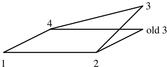
The standard technique is to divide the square formed by rows and columns into two triangles because, not only are three points guaranteed to be in the same plane, the three points define the plane.
