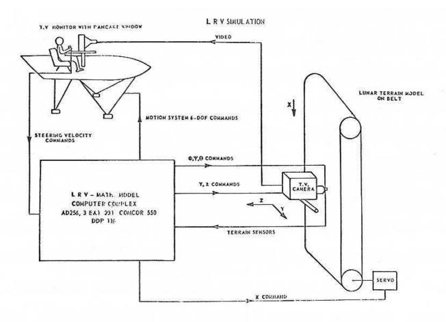
The SMK-23 used a television camera with an optical probe to fly over the terrain model contained on a servo-driven endless belt.
