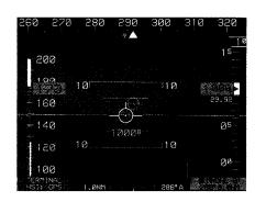
using HITS in Juneau, Alaska, on Mar. 31. It followed an optimized area navigation (RNAV) route through airspace that would be inaccessible with conventional avionics.
