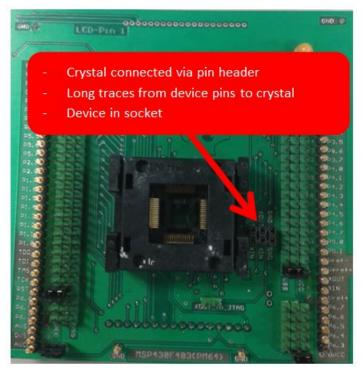
Figure 11. Nonoptimized PCB for General Test Purpose
