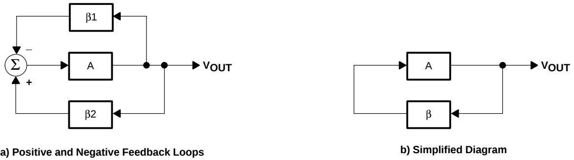
Figure 5. Block Diagram of an Oscillator
